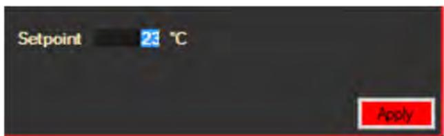
Figure 7 Apply button appears when settings are changed
