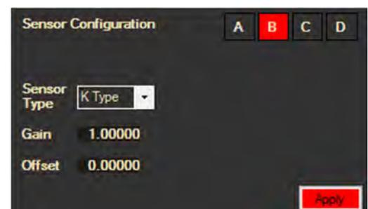
Figure 24 Selection of a K type thermocouple from the sensor configuration page
