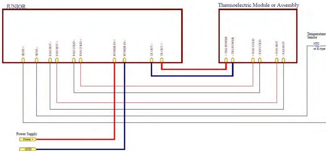
**Figure 3a. Wiring diagram of minimum level installation**
