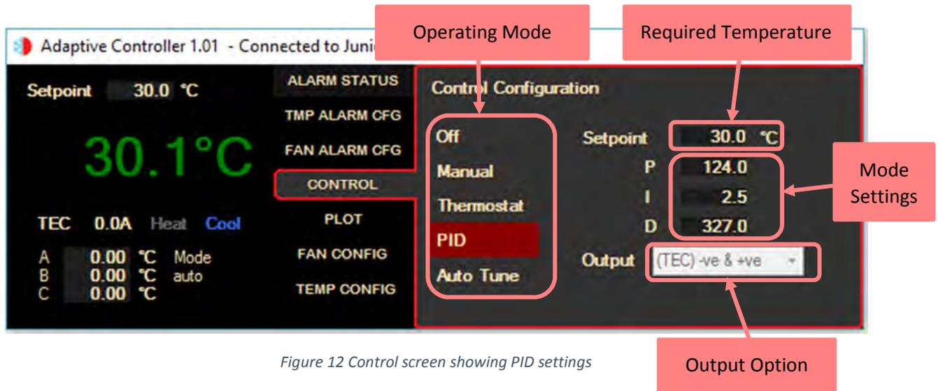
Figure 12 Control screen showing PID settings
