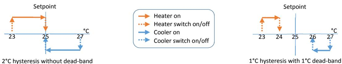
Figure 16 Example configuration shown hysteresis and dead-band for bidirectional drive
