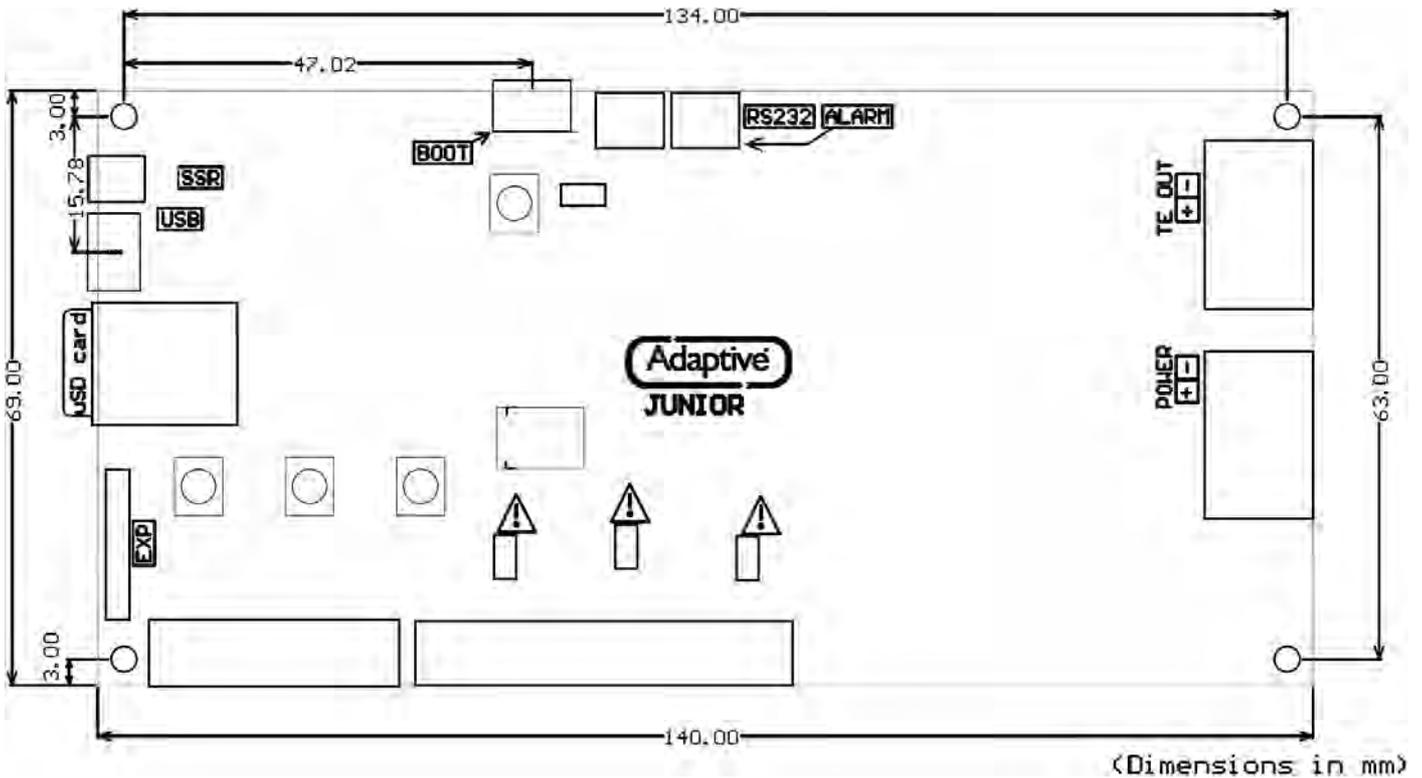
Figure 5. Mechanical Dimensions
