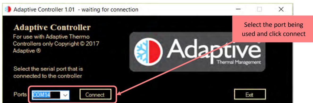
Figure 8 HMI connection screen
