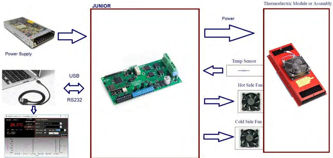
**Figure 2. Thermoelectric Cooling / Heating Application Setup**
