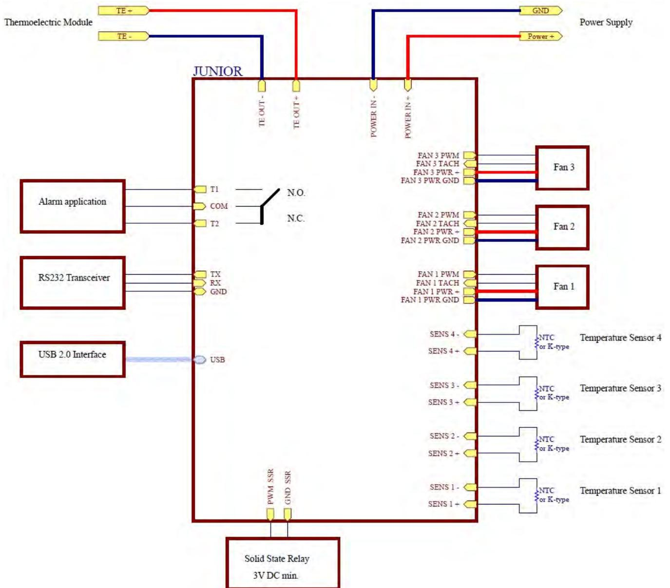
Figure 3b. Wiring diagram of complete installation
