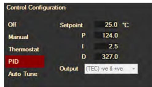
Figure 17 PID Operating mode
