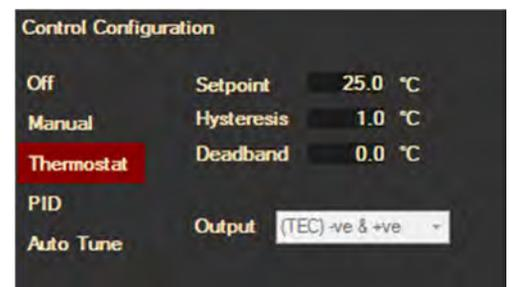
Figure 15 Thermostat operating mode
