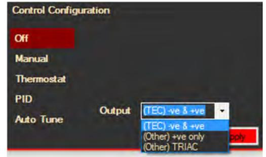
Figure 14 Selecting the output drive method when the control mode is OFF
